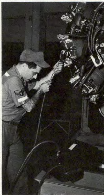
Cylinder compression tests reveal ring or valve failure.
