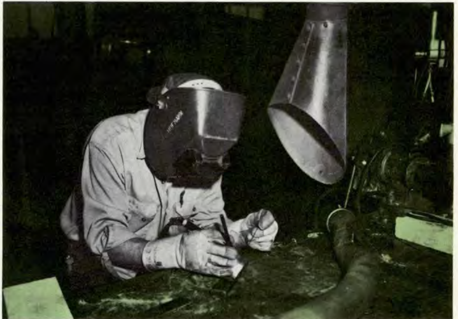
Proper venting is essential for heliarc welding in confined areas.
