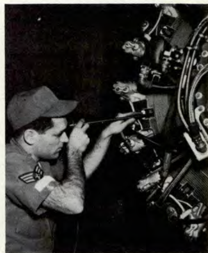
Borescoping is effective method for detecting internal failure.
